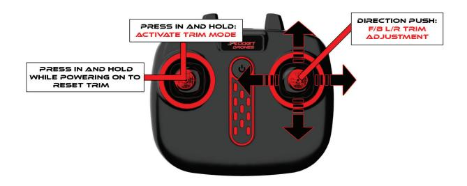
To reset the trim, press and hold the left stick while powering on the controller.
